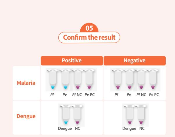
Amplified targets can be confirmed by identifying color change of solution without using any additional devices. When the specific target is amplified, the color of the solution shows a blue color.
